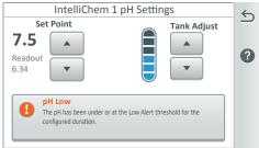
**ph Reading/Set Point/Tank:** Displays the current pH level reading. Tap the **Set Point Up/Down button** to adjust the pH set point value. The adjustable range is from 7.2 to 7.6 in increments of 0.1. The default pH set point value is 7.5.
