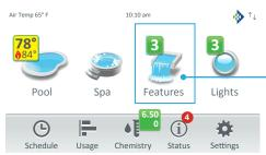
Green Number Badge: Displays the number of active feature circuits. Tap the Features icon on the Home screen to display the Feature circuits. To hide the Features number badge. See page 57, Settings > Advanced System Configuration > Installation Setup > Circuits > Feature Circuits > Feature Circuit Settings (Visible in Features (Y/N) option).
