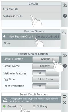
+ New Feature Circuit (Generic or Spillway): Tap New Feature Circuit to create a new Feature Circuit (up to 32 total). Select the Feature Circuit Name, from the displayed list or tap the Keyboard icon and enter a custom name.
