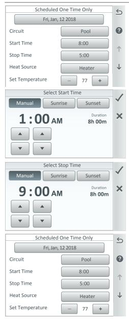
**Don't Change Heat Source:** Don't Change is only used when a schedule is running. The heater source selected from the Pool or Spa screen will be used every time the schedule is active. See page 9. Start Time (Manual): Set the start time (am/pm) for the Weekly schedule.
