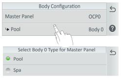
**Pool (Body 0 Settings):** From this screen you can reassign the body type/\*, name and capacity.
