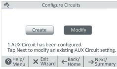
**Create / Modify:** Tap **Next** after the first AUX Circuit has been configured. The Configure Circuits screen is displayed. Select either **Create** or **Modify** to create a new circuit or modify an existing AUX Circuit. After you have configured all of the available AUX Circuits, tap **Next** to continue to Feature Circuits.
