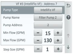
**Minimum Flow (GPM):** The pump's minimum flow rate can be set from 15-130. This is the minimum flow rate speed but still generating sufficient flow in the pool. The IntelliCenter<sup>®</sup> Control System will not run lower than 15 GPM. The lower you can establish this flow rate the better the energy savings.
