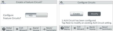
**Create / Modify:** Tap **Next** after the first AUX Circuit has been configured. The Configure Circuits screen is displayed. Select either **Create** or **Modify** to create a new circuit or modify an existing AUX Circuit. After you have configured all of the available AUX Circuits, tap **Next** to continue to Configure Valves.
