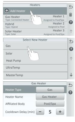
Add Heater: Tap Add Heater to add a new heater type. Up to three heaters can be assigned. Note: Only one gas heater for each body of water. For shared equipment; one gas heater (pool/spa).
