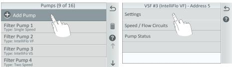
IntelliFlo VSF Settings: Pump Type, Name, Address, Min. Speed (450 RPM), Max. Speed (3450 RPM), Min. Flow (GPM 20 GPM), Max. Flow (140 GPM), Step Size (10-250 RPM), and Step Size (1-10 GPM). For information about priming the pump, see page 70.
