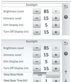
**Back Light:** Brightness Level: Adjust the screen brightness level from 33 to 100%.
