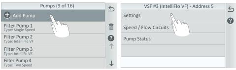
IntelliFlo VF Settings: Pump Type, Pump Name, Pump Address, Min. Flow (15 GPM), Max. Flow (130 GPM), and Step Size (1-10 GPM). For information about priming the pump, see page 70.
