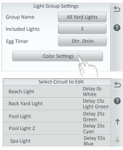
**Color Settings:** Tap this button to display the assigned light circuits and the current delay time and selected light color.
