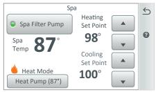
**Spa Heater Button:** Tap to access the Select Heat Mode screen. Tap the desired heat source (solar or conventional heaters). Note: Heat sources are configured from Settings > Advanced System Configuration > Installation Setup > Circuits, see page 56. Also see: Manual OP Priority: Manual ON/OFF circuit during a schedule. See page 44.
