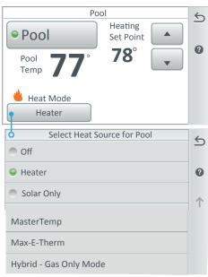
Heat Mode: Heat Pump Only: Uses only the Heat Pump side during calls for heating. Hybrid - Gas Only Mode: Use only the Gas Heater side during calls for heating. Hybrid - Hybrid Mode: Uses Gas and/or Heat Pump (automatically switches) depending on conditions during calls for heating. Hybrid - Dual Mode: Heat Pump and Gas Heater will run in tandem during calls for heating. Provides fastest possible heat ups. Note: To add a heater, see page 72.
