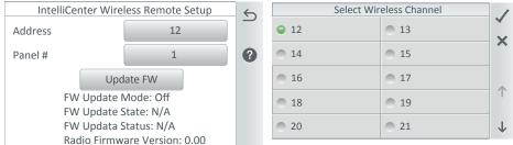
Address: Display the current wireless channel being used. For most operations address 15 is the default address. If you should need to change the address, tap the Address button to access the Select Wireless Channel screen and select a different channel from 12 through 25. The unique wireless address communicates to the wireless transceiver located at the IntelliCenter Control System load center.
