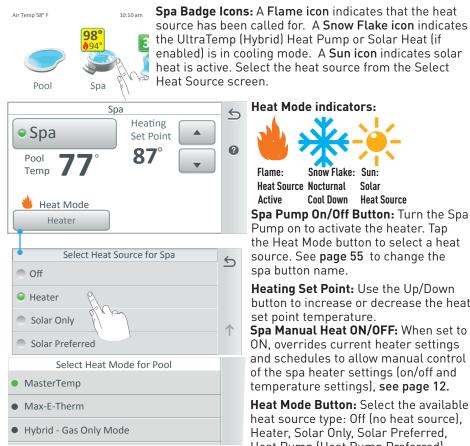
Heat Mode: Heat Pump Only: Uses only the Heat Pump side during calls for heating. Hybrid - Gas Only Mode: Use only the Gas Heater side during calls for heating. Hybrid - Hybrid Mode: Uses Gas and/or Heat Pump (automatically switches) depending on conditions during calls for heating. Hybrid - Dual Mode: Heat Pump and Gas Heater will run in tandem during calls for heating. Provides fastest possible heat ups.
