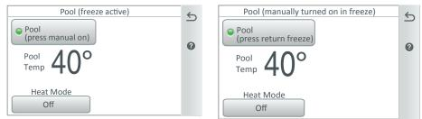
**Freeze Protection Override:** The pool pump can be manually turned on to override the Freeze protection. This also applies if a schedule is running. To assign freeze protection to a circuit. **See page 59 for more information.**
