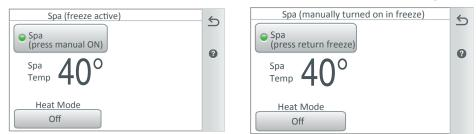
**Spa Freeze Override Time (0-240 min (4 hrs):** Override the spa pump circuit that has freeze protection active to run the pump and heat the spa during freezing temperatures. This also applies if a schedule is running. **Freeze Cycle Time (min):** Set the freeze protection time from 5 to 60 minutes to run the pump during freezing temperatures. Default time is 5 minutes. **See page 88 and 59.**
