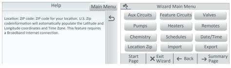
Help Screen/Main Menu Button: From any of the Wizard Setup screens, tap Help to display the help text. Tap the Main Menu button to display the Wizard Main Menu items. Main Menu: Tap the Main Menu button on the Help text screen to display the Main Menu items. Also, tap and hold and release the Help/Main Menu button on any of the Wizard Setup screens to display the Main Menu items. Start Page: Return to the first Wizard
