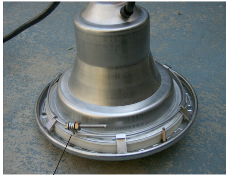
Spring clamp: Remove nut and screw
