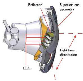
Drawing shows unique lens and reflector designs which combine to provide superior light beam distribution.
